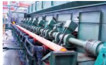
Pipe-body Heat Treatment
